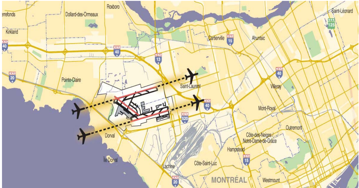
Northeasterly/easterly winds (30% of the time) Runways 06 for takeoff and landings
